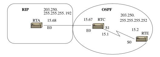
In the above diagram, RTE is running OSPF and RTA is running RIP. RTC is doing the redistribution between the two protocols. The problem is that the class C network 203.250.15.0 is variably subnetted, it has two different masks 255.255.255.252 and 255.255.192. Let us look at the configuration and the routing tables of RTE and RTA:
