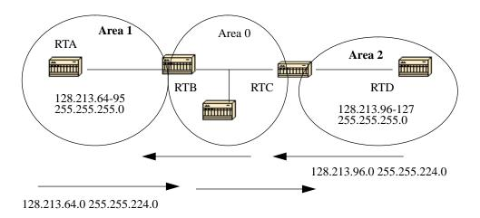
In the above diagram, RTB is summarizing the range of subnets from 128.213.64.0 to 128.213.95.0 into one range: 128.213.64.0 255.255.224.0. This is achieved by masking the first three left most bits of 64 using a mask of 255.255.244.0. In the same way, RTC is generating the summary address 128.213.96.0 255.255.224.0 into the backbone. Note that this
