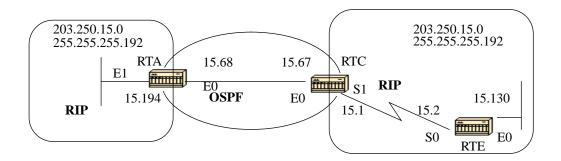
To illustrate, suppose RTA, RTC, and RTE are running RIP. RTC and RTA are also running OSPF. Both RTC and RTA are doing redistribution between RIP and OSPF. Let us assume that you do not want the RIP coming from RTE to be injected into the OSPF domain so you put a passive interface for RIP on EO of RTC. However, you have allowed the RIP coming from RTA to be injected into OSPF. Here is the outcome (DO NOT USE THE FOLLOWING CONFIGURATION):
