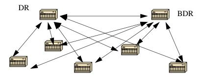
In the above diagram, all routers share a common multi-access segment. Due to the exchange of Hello packets, one router is elected DR and
