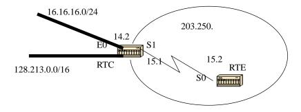
Suppose we added two static routes pointing to E0 on RTC: 16.16.16.0 255.255.255.0 (the /24 notation indicates a 24 bit mask starting from the far left) and 128.213.0.0 255.255.0.0. The following shows the different
