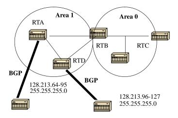
In the above diagram, RTA and RTD are injecting external routes into OSPF by redistribution. RTA is injecting subnets in the range 128.213.64-95 and RTD is injecting subnets in the range 128.213.96-127. In order to
