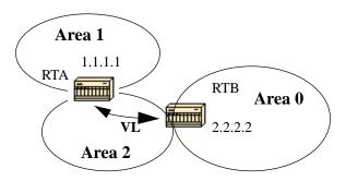
In this example, area 1 does not have a direct physical connection into area 0. A virtual link has to be configured between RTA and RTB. Area 2 is to be used as a transit area and RTB is the entry point into area 0. This way RTA and area 1 will have a logical connection to the backbone. In order to configure a virtual link, use the following router OSPF subcommand on both RTA and RTB:
